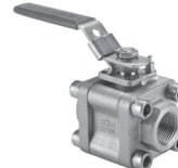
3-Piece Maintenance Design *Style BVM3 Class 800 1920 W.O.G. R-PTFE Seats Sizes 1/4" - 2 1/2" Full & Reduced Port
