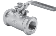
Seal Welded *Style BVS3 Class 1500 (3600 PSIG) Delrin AF Seats Sizes 1/4" - 2" Full & Reduced Port
